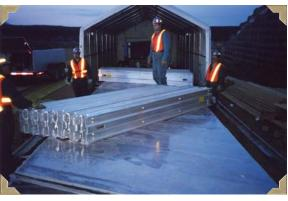
The unique Almex flexible platen, pressure bag and temperature control system provided uniform pressure over the entire splice area giving the strongest splices.
