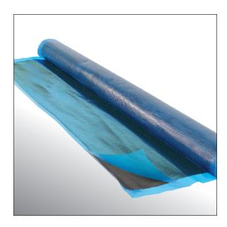
Steel Cord Belt Cable Gum is an uncured rubber for hot vulcanized belt splicing. It is designed to use as an inter-core cord rubber replacement material in splicing steel cord conveyor belts or a tie gum in fabric belts. This material is designed to bond to cured inter-core rubber and wire cords in all standard grade steel cord conveyor belts. Use Steel Cord Belt Cable Gum for fabric belt cured skim rubber and general bond improvement material for general grade fabric conveyor belts.
