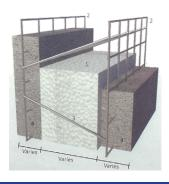
RSG 3-D Panel is a lightweight Panel consisting of continuous EPS insulation, incorporating a proprietary steel truss-system and welded wire fabric. The Panels are easily and rapidly framed. EMP roughs-in quickly and accurately. Then the Panels receive a field-applied concrete finish.
