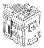
2 Insert the AXS memory card into the card slot with the label facing as indicated below.
