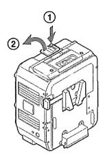
Insert the projection of the AXS-R5 into the slot on the rear of the camcorder (1), then lower the ejection lever (2).
