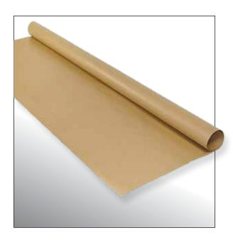
Almex Silicone Treated Release Paper is a calendered Kraft-type paper with a special rubber flow enhancing coating. It is designed to be used as a release material between the uncured rubber and vulcanizing press. It can be used in step splicing, finger splicing and steel cord splicing of all types of belts.
