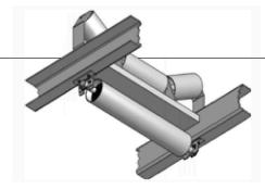
Belts must always run straight on all conveyors. Belts can mistrack, often without any known reason. When the belt mistracks the force and belt weight make the roll tilt and turn thanks to the Prime Pivot bush. The belt will have full contact with the tracker.
