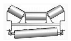
A cylindrical tracker has the same peripheral speed over the whole surface. A crowned roll has different speeds at its center and roll edges. Using a crowned roll may result in insufficient belt guidance and worn out roll ends. This is why Prime Tracker is cylindrical.
