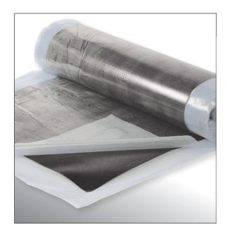
Fabric Belt Cover Stock is an uncured rubber used in hot vulcanized belt step and finger splicing. It is designed for use as a cover rubber replacement material when splicing fabric conveyor belts. A high abrasion compound, it will to bond to cured cover rubber in all standard grades of fabric conveyor belts.
