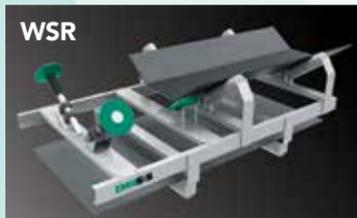
The EMSYS WSR uses RFID Technology to provide a reference point and the belt is then operated for several revolutions. Measurements are taken every few centimeters and the WSR system learns the width of the conveyor for its entire belt length as a baseline. If the belt is ripped, the width of the belt will change and trigger a signal and/or stop the belt.
