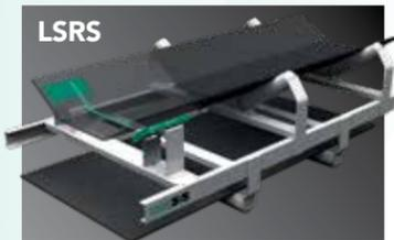
The EMSYS LSRS monitors the belt via embedded wires that can detect rips and damage to the belt through SmartWire technology. The LSRS will read most major belt manufacturers rip detection loops and antennae. SmartWire can be embedded in a newly manufactured belt or retrofit into an existing belt in under an hour.
