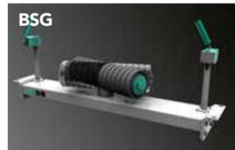
EMSYS offers the Belt Steering Gear (BSG) system to provide precise belt alignment control and monitoring of the belt tracking, onsite or remotely via an application on your phone or tablet. A combination of an actuator and sensors and idlers before and after this sensor can detect and correct any belt misalignment, even remotely.
