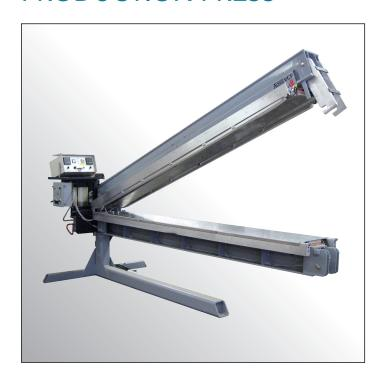
The Cantilever VCF Press is the superior press for splicing lightweight rubber conveyor beligng. With increased pressure capacity, the Cantilever VCF is designed for rubber conveyors that do not require heavyweight splice equipment
