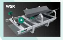
The EMSYS WSR uses RFID Technology to provide a reference point and the belt is then operated for several revolutions. Measurements are taken every few centimeters and the WSR system learns the width of the conveyor for its entire belt length as a baseline. If the belt is ripped, the width of the belt will change and trigger a signal and/or stop the belt.
