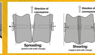
When a conveyor belt is ripped due to a foreign object it will
